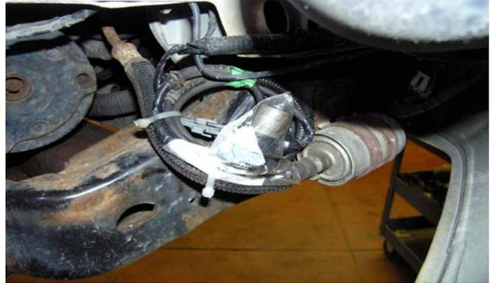
**FIG 3, Strut Solenoid Removed**
