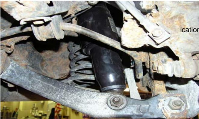
**FIG 10, Rear Shock Installed Upper Portion Right Side**
