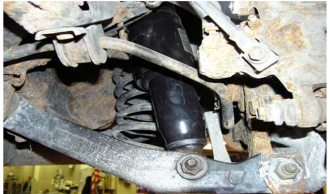
FIG 10, Rear Shock Installed Upper Portion Right Side
