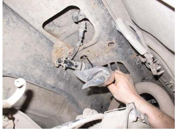
FIG 5, Ride Height Sensor secured Solenoid Tucked
