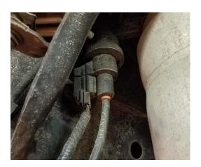
6. To remove the air strut assembly, remove the lower strut mount bolt at the lower control arm. Save bolt for reuse. Disconnect the lower end of the ride height sensor link from the lower control arm. Next, remove the lower inner control arm to frame bolt and nut. Pry down on the lower control arm and pivot out of the way. Support the air strut by the lower mount.
