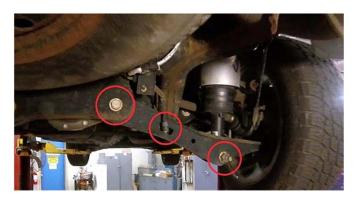
7. Next remove the three (3) upper mounting nuts and the air strut assembly from the vehicle.
