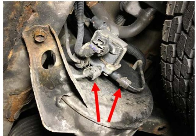
5. Remove the air spring assembly along with the air line.
