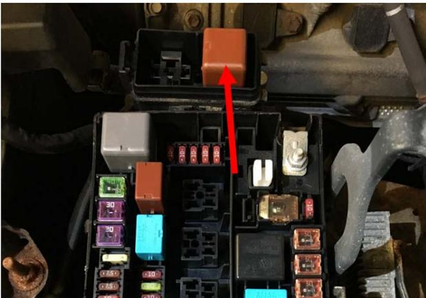
13. Remove the 20 amp TEMS fuse located in the driver side junction box near the lower left end of dash. This will prevent the height control portion of the instrument panel from illuminating.
