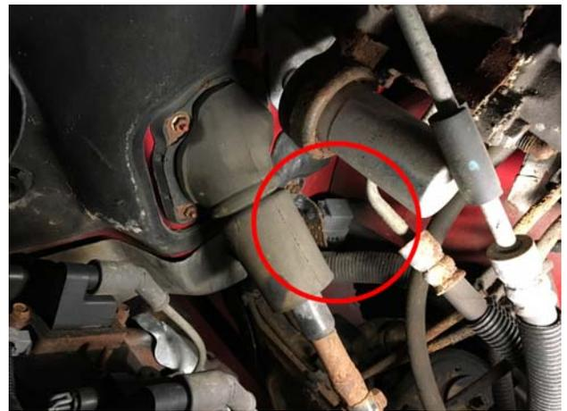
16. Locate the 24-pin connector for the air suspension module. It is located at the rear of the vehicle, near the trailer hitch, and behind the rear differential housing. Remove the red plastic retaining clip and then the 24-pin connector. Place the remaining bag and zip tie over the connector to protect from contaminants.
