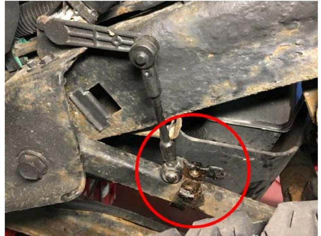
6. Remove the bolt that holds the brake line bracket to the rear differential.
