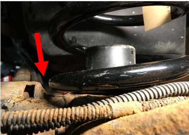
11. Carefully raise the rear axle while ensuring the upper coils remain properly seated in the upper spring seats. **Caution:** *Take care that vehicle weight does not shift off frame supporting points when lifting the axle.*
