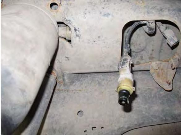
FIG 3, Solenoids and Ride Height Sensor
