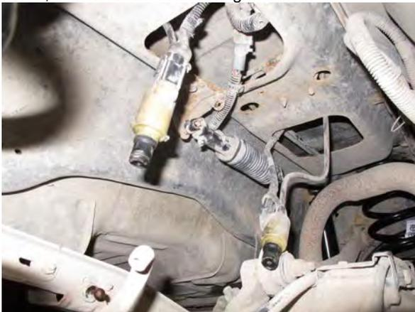
FIG 4, Solenoid packaged and ready to tuck into frame pocket
